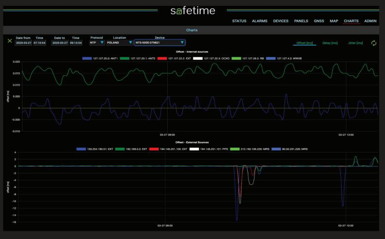
Plotting charts is one of major functionalities. Multiple servers can be observed simultaneously for all 3 parameters: OFFSET to UTC, network DELAY, synchronization JITTER. It lets administrator compare beehive of time servers located in different places but measured from one common point of reference – the central management system.
