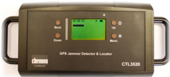
Figure 18 Device identifying jamming and showing the direction of its source
